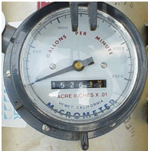
Figure 3. Image of a water meter counter showing the ending irrigation volume used in the example and the dial used for instantaneous flow. Photo courtesy of GSWCC.
